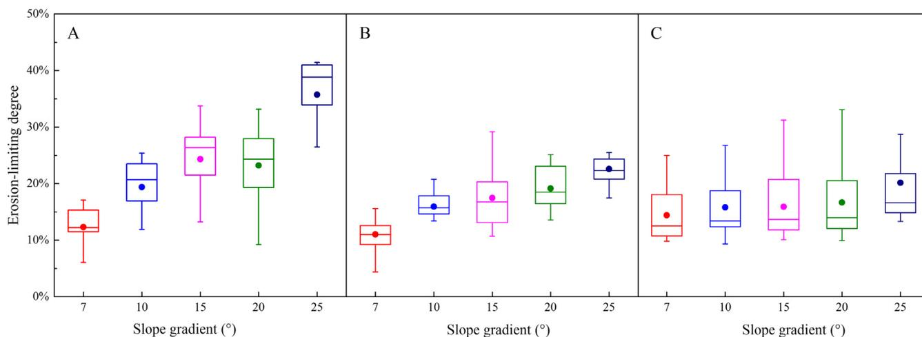
Fig. 6. Box-plots of erosion-limiting degree at low rainfall intensity (A:  $42 \text{ mm h}^{-1}$ ), moderate rainfall intensity (B:  $60 \text{ mm h}^{-1}$ ) and high rainfall intensity (C:  $90 \text{ mm h}^{-1}$ ).
