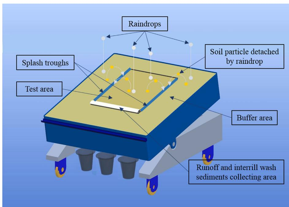
Fig. 1. Soil erosion pan used in this study.
