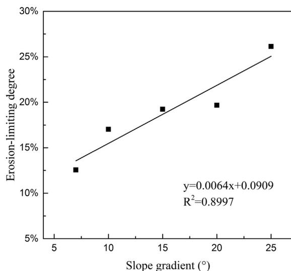
Fig. 7. Relationship between erosion-limiting degree and slope gradient.
