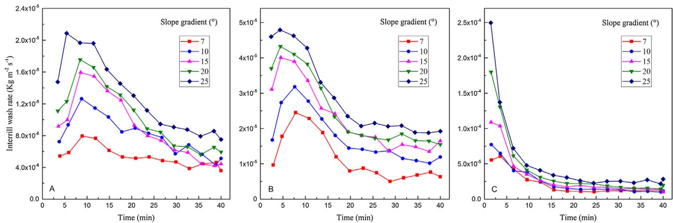
Fig. 4. Temporal variations of interrill wash rate under different slope gradients at low rainfall intensity (A: 42 mm h<sup>-1</sup>), moderate rainfall intensity (B: 60 mm h<sup>-1</sup>) and high rainfall intensity (C: 90 mm h<sup>-1</sup>).
