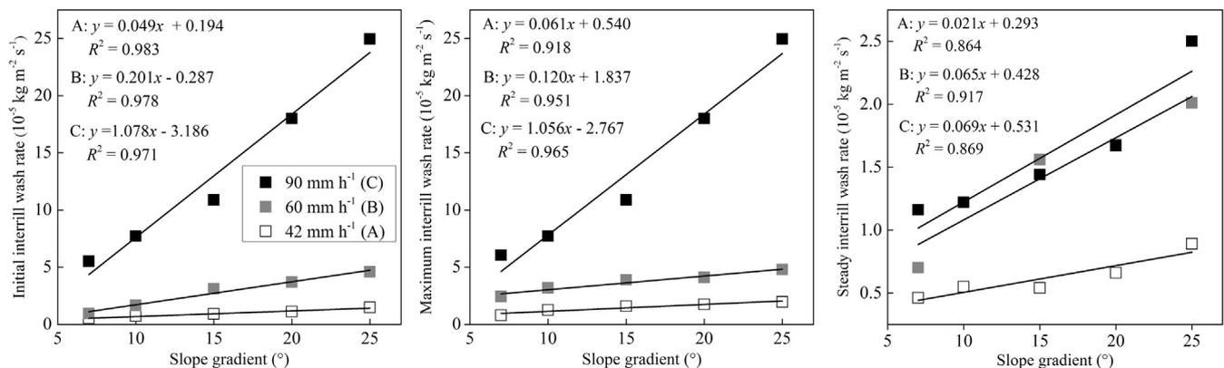
Fig. 5. Variations of initial interrill wash rate, maximum interrill wash rate and steady interrill wash rate with slope gradient under different rainfall intensities.
