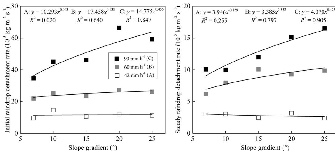
Fig. 3. Variations of initial raindrop detachment rate and steady raindrop detachment rate with slope gradient under different rainfall intensities.
