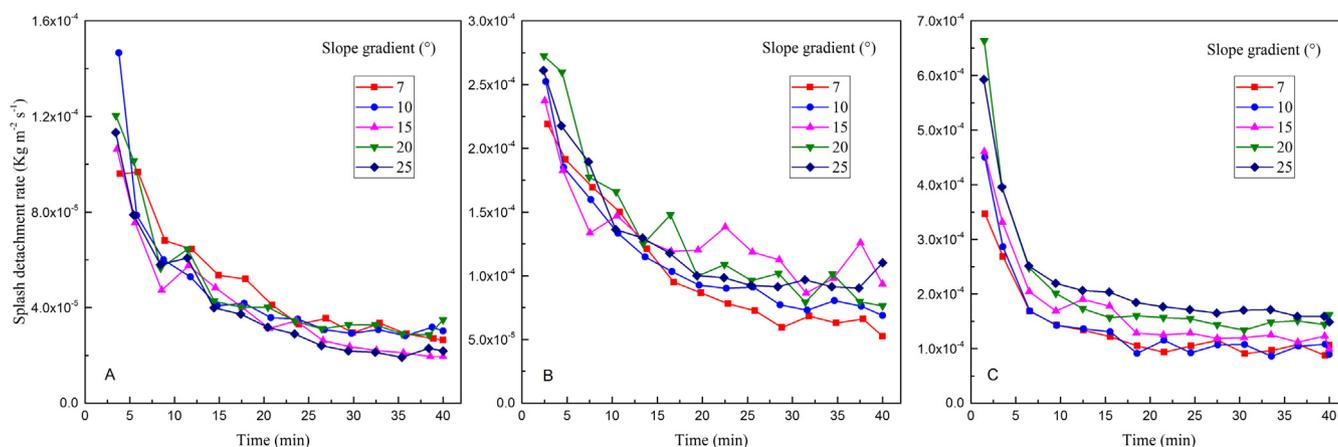
Fig. 2. Temporal variations of raindrop detachment rate under different slope gradients at low rainfall intensity (A: 42 mm h<sup>-1</sup>), moderate rainfall intensity (B: 60 mm h<sup>-1</sup>) and high rainfall intensity (C: 90 mm h<sup>-1</sup>).
