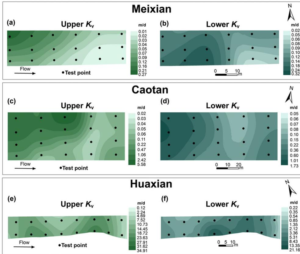
**FIGURE 8** Interpolated contour maps of  $K_v$  in the upper and lower layers for each test site along the Weihe River: (a,b) Meixian site, (c,d) Caotan site, and (e,f) Huaxian site. The test location is shown in Figure 1f–h
