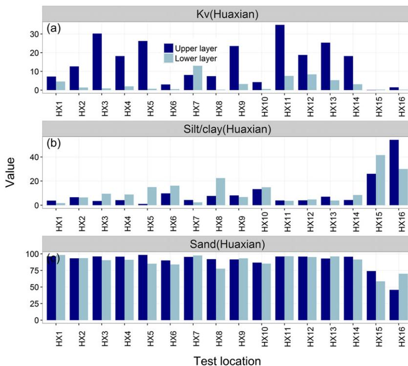
**FIGURE 7** The bar plots of the (a)  $K_v$  value, the contents of (b) silt/clay, and (c) sand in the upper and lower layers of sediments at each location of the Huaxian site. All  $K_v$  magnitudes are in metres per day. The magnitudes of all contents of silt/clay and sand are in percent
