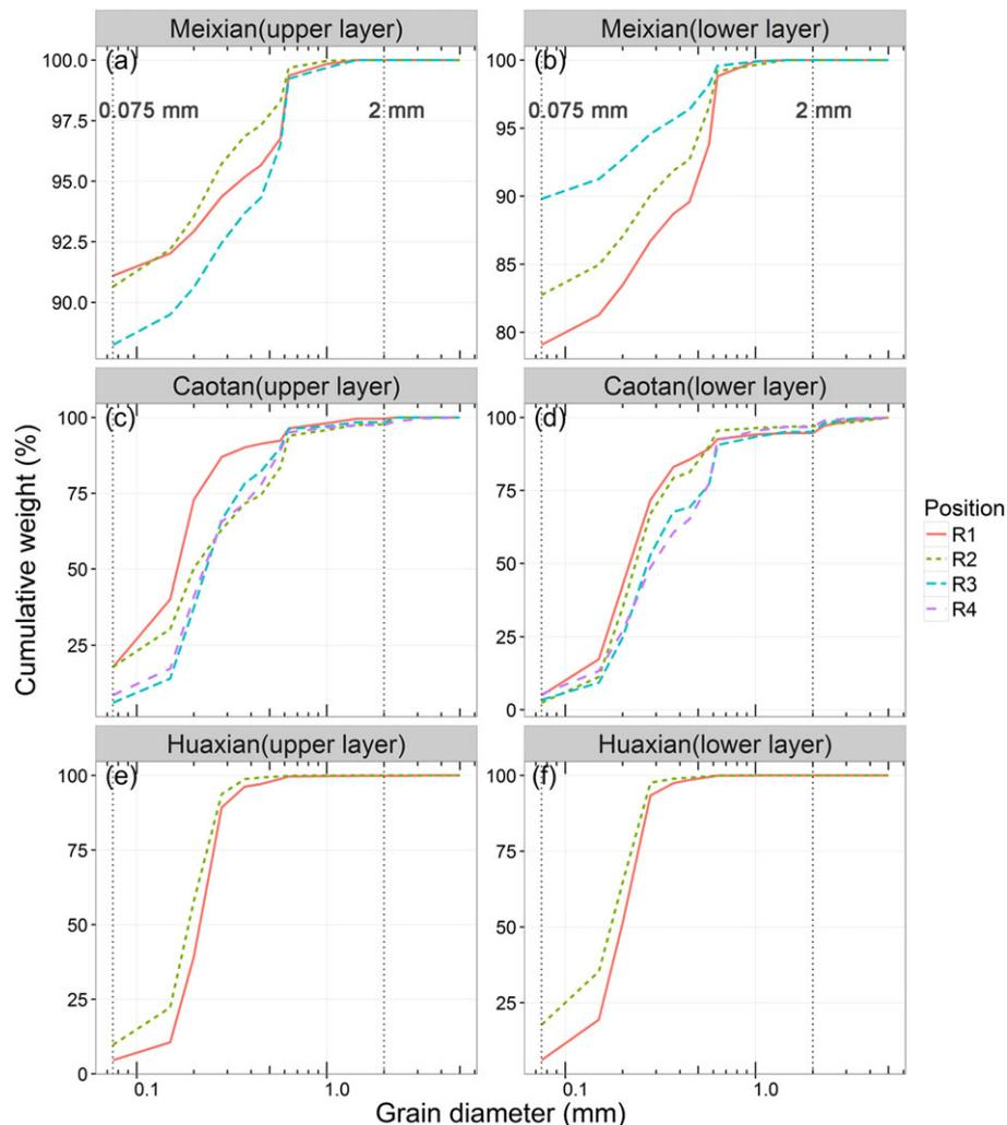
**FIGURE 11** The grain size distributions of streambed sediment cores for each position across the stream from (a) the upper layer of the Meixian site, (b) the lower layer of the Meixian site, (c) the upper layer of the Caotan site, (d) the lower layer of the Caotan site, (e) the upper layer of the Huaxian site, and (f) the lower layer of the Huaxian site
