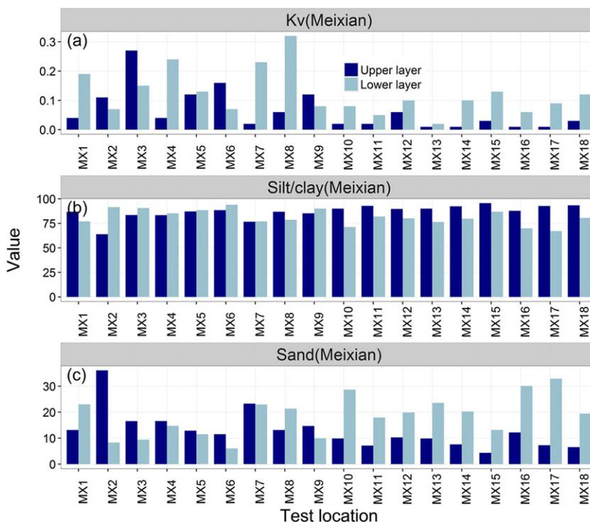
**FIGURE 5** The bar plots of the (a)  $K_v$  value, the contents of (b) silt/clay, and (c) sand in the upper and lower layers of sediments at each location of the Meixian site. All  $K_v$  magnitudes are in metres per day. The magnitudes of all contents of silt/clay and sand are in percent
