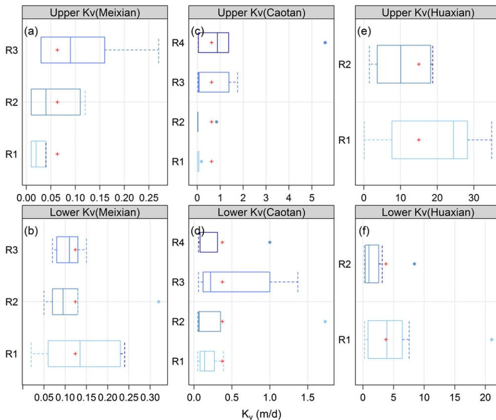
**FIGURE 9** Box plots of  $K_v$  in the upper and lower layers for each position across the stream at each test site: (a,b) Meixian site, (c,d) Caotan site, and (e,f) Huaxian site. All  $K_v$  magnitudes are in metres per day. + indicates the mean value. \* indicates outliers
