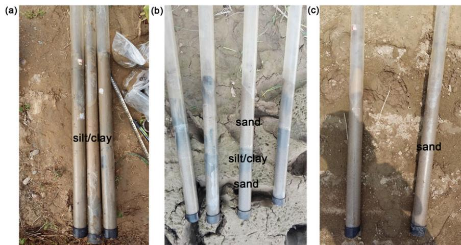
**FIGURE 2** Typical cores of (a) mainly uniform silt and clay or (b) sand with a continuous silt and clay layer or (c) sand without silt and clay layer. The cores shown on the pictures are test locations (a) MX10–MX12, (b) CT13–CT16, and (c) HX3–HX4
