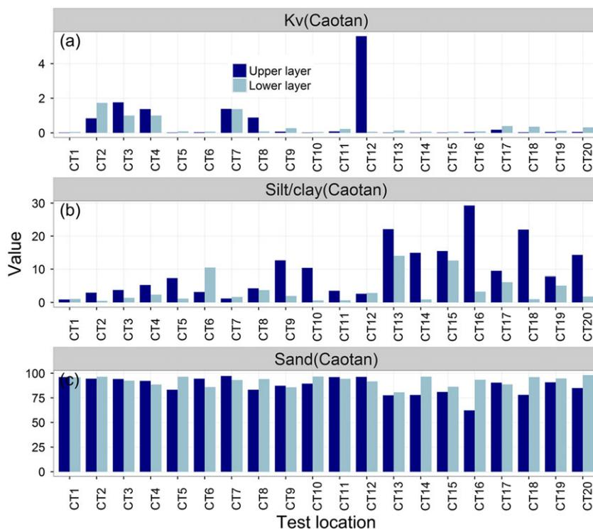
**FIGURE 6** The bar plots of the (a)  $K_v$  value, the contents of (b) silt/clay, and (c) sand in the upper and lower layers of sediments at each location of the Caotan site. All  $K_v$  magnitudes are in metres per day. The magnitudes of all contents of silt/clay and sand are in percent
