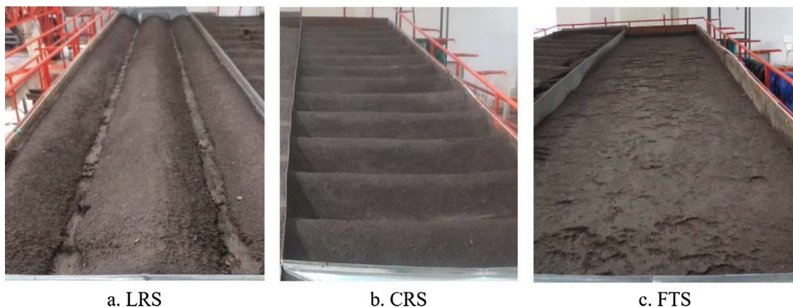
Fig. 3. Different tillage systems. Notice that photos of LRS and FTS (a and c) are taken after rainfall test to show the erosion morphology while photo of CRS (b) was taken before test.
