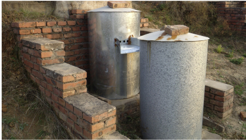
Fig. 1. The arrangement of collection buckets at the lower outlets of the experimental plots.
