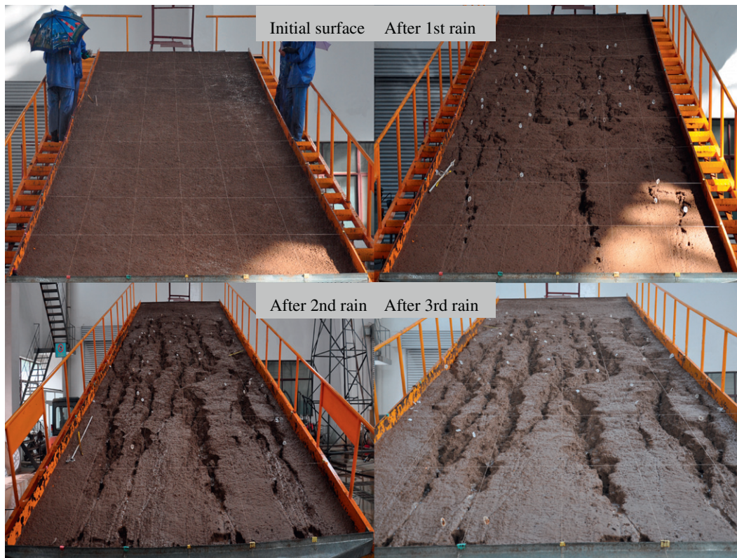
Fig. 2. Initial surface and rill networks after each rain at the 50 \text{ mm h}^{-1} rainfall intensity.
